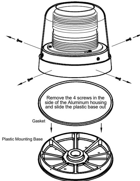
1. Remove the four screws in the side of the aluminum housing.
