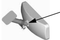
8. Attach the clamp to the bracket with the washer, nut and bolt, securing your light to the rear view mirror.
