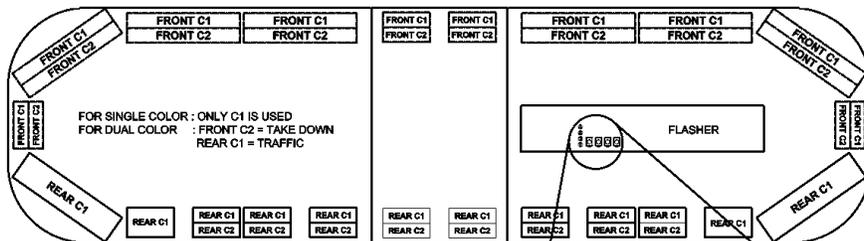
Advanced programming of this lightbar is done using four (4) pushbuttons and 4 LEDs located on the circuit that is installed on the right side of the lightbar (facing front).
