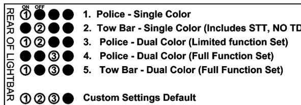
3. Press the Program button once and compare the flickering LED display on the circuit board with the diagram to the right to determine which default was last used (note: the user may have reprogrammed some options).
