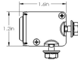
We also include two L-Brackets to facilitate mounting. These are optional and do not need to be used.
