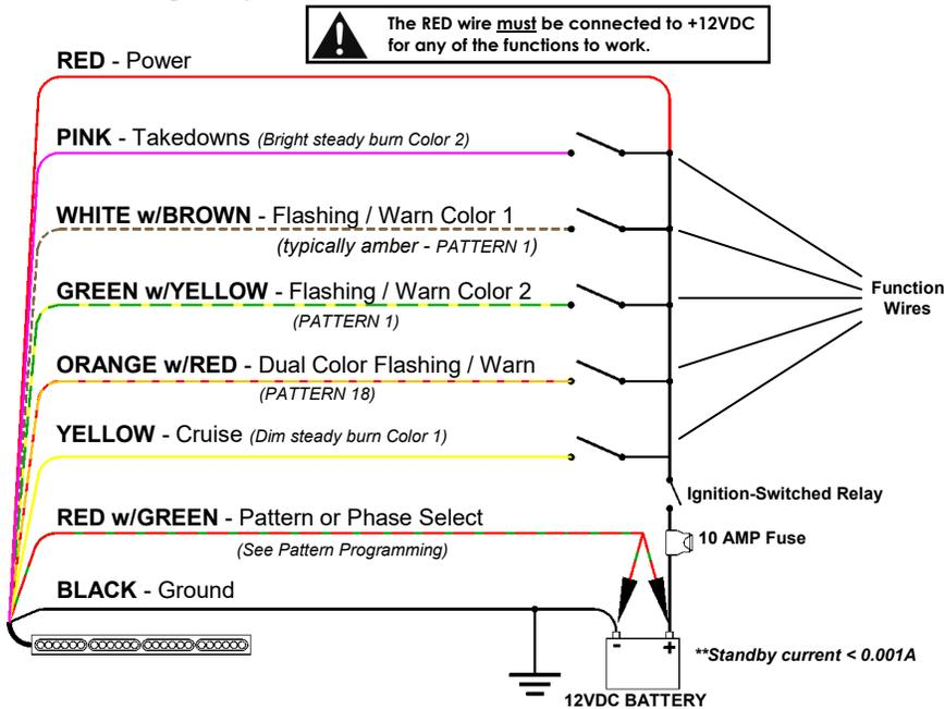
**Note:** The wires are shown above in order of Priority. Higher priority wires will override the patterns on any lower priority wires for the heads that are enabled.
